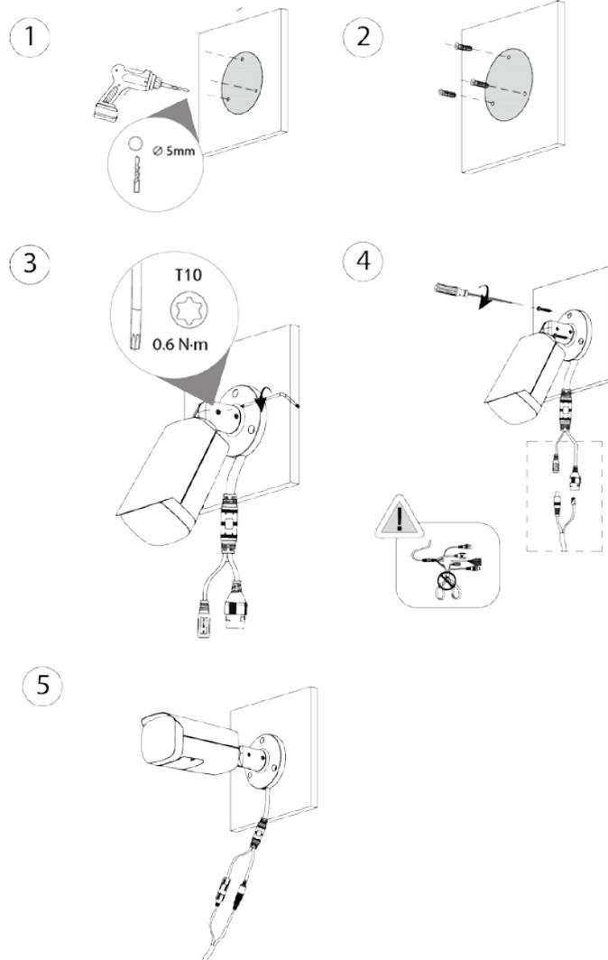
Figure 3-8 Cable going through the mounting surface
