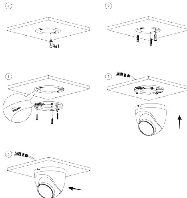
Figure 3-8 Cable going through the side cable tray
