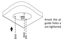
Knock the plastic rivets into the guide holes and ensure that they are tightened up.
