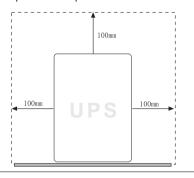
The UPS is intended for indoor use only. Although your UPS is very rugged, its internal components are not sealed from the environment, Kindly note the following.
