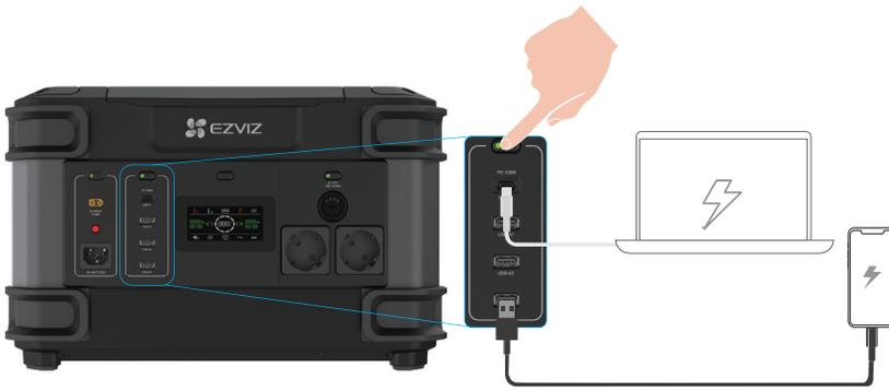
After using the power station, Please disconnect the wires on the power station, and press to turn off the USB output button to save power.
