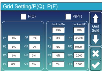
**P(Q)**: It is used to adjust the inverter reactive power according to the set active power.
