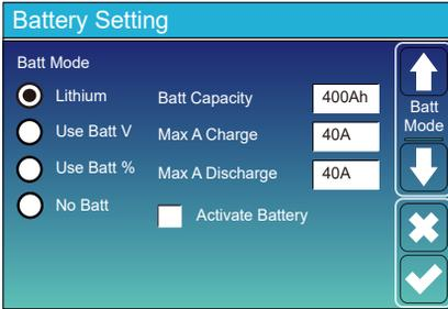
**Battery capacity:** it tells Deye hybrid inverter to know your battery bank size.
