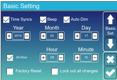
**Factory Reset:** Reset all parameters of the inverter.
