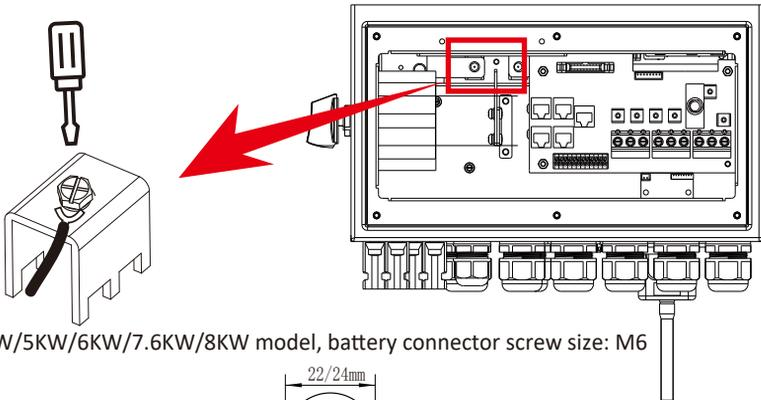
For 3.6KW/5KW/6KW/7.6KW/8KW model, battery connector screw size: M6
