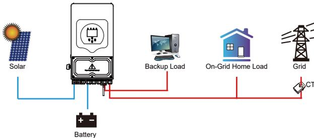
**Solar Sell:** "Solar sell" is for Zero export to load or Zero export to CT: when this item is active, the surplus energy can be sold back to grid. When it is active, PV Power source priority usage is as follows: load consumption and charge battery and feed into grid.
