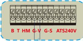
GV/GS: dry contact signal for startup the diesel generator.
