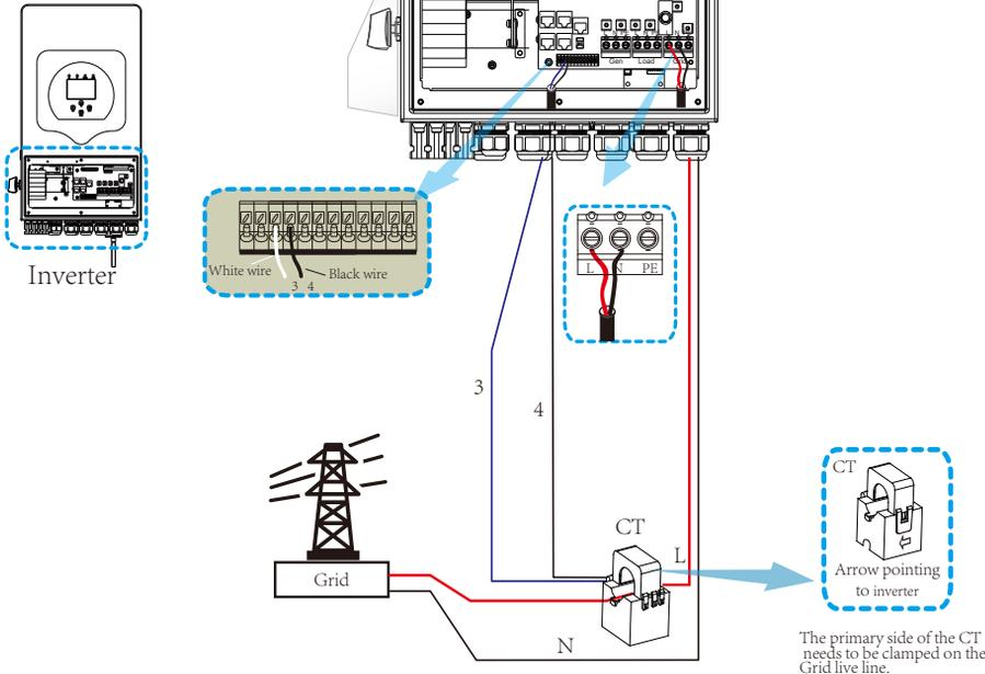
**\*Note:** when the reading of the load power on the LCD is not correct, please reverse the CT arrow.
