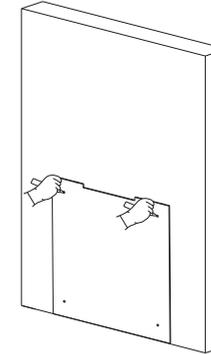
3. Drill 2 holes on the wall with a diameter of 10mm and a depth of about 70mm.
