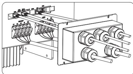
Installation method of two communication cables via M25 cable gland
