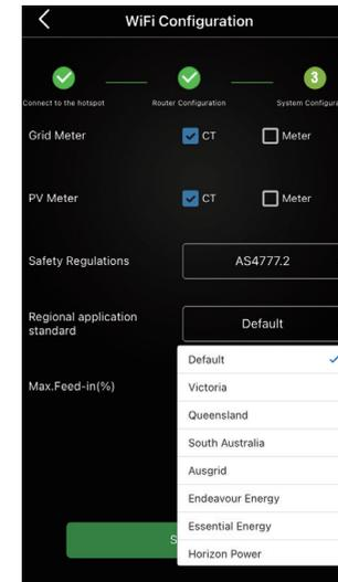
**Step 5:** Set basic parameters, including PV capacity on the grid side, the type of meters, safety regulations and regional application standard. Click "Submit" when the settings are complete.
