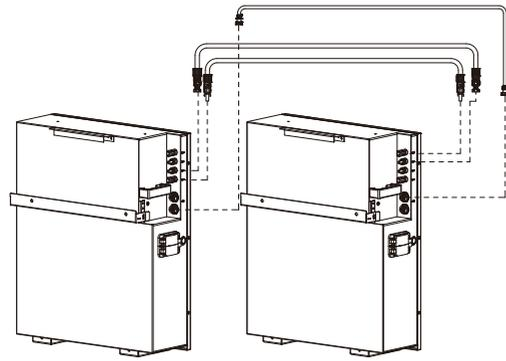
Install extra batteries by side, without stack
