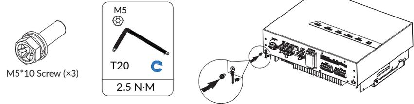
An external grounding connection is provided at the left side of battery pack. Prepare and connect grounding connection as above. The Battery Pack and the inverter need to be grounded.
