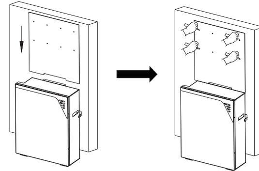
2. Cover the top of the battery with plastic bag and drill 4 holes on the wall with drill 10, insert 4 screw anchors into the drill holes.
