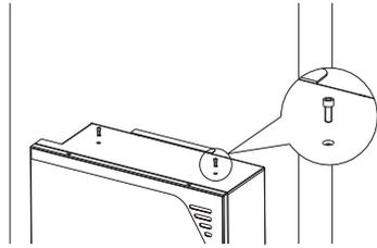
For Battery Pack (OUTDOOR) stack, lock the foot pad on top of the first battery pack.
