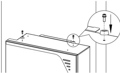
The bottom limit holes of the second battery will match the top screws (or foot pad) of the first battery.
