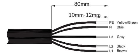
4. Insert the stripped part of the conductors into the cord end terminals and crimp them using a crimping tool.
