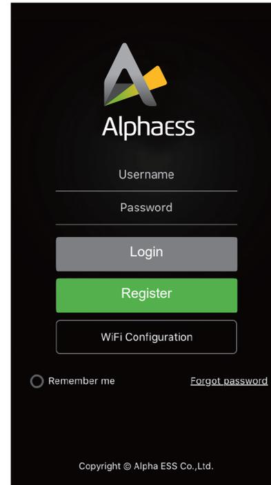
**Step 1:** Open AlphaESS APP, click the “Wi-Fi Configuration” button and enter the WiFi configuration interface.
