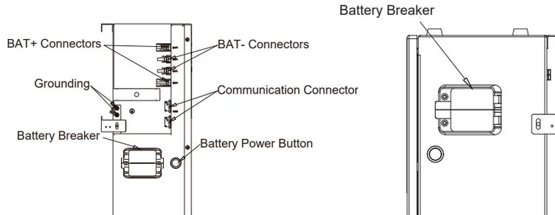
The battery breaker is switched off when shipped.
