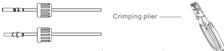
Pic 3.13 Crimp the contact pin to the wire
