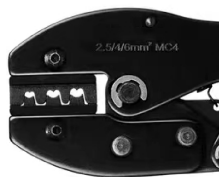
Crimping die for cold forming contact
