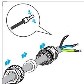
Step 3: Establish connections between L1, N, and PE.
