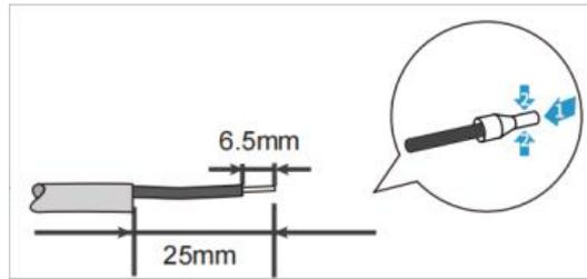
Step 2: Connect the communication signal cables, such as batteries and meters, to the BAT-COM plug in the correct position. (Tighten with the proper tool. Please find the tools in the accessory box in the packing box.)
