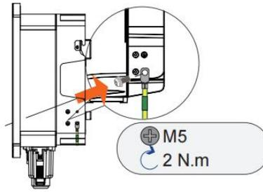
Step 3: Apply paint to the grounding terminal to ensure corrosion resistance.
