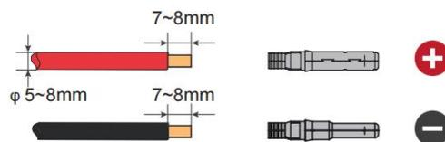
Step 2: Assembling the Crimp contact and cable, use the crimping pliers to securely assemble the cable ends.
