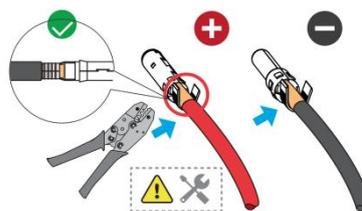
Step 3: Lead the cable through the cable gland and insert the crimp contact into the insulator until it audibly
