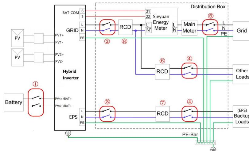
Note: All the home load can be connected to the EPS line as backup load, when the total amount of the load less than 6kW. If 6kw is exceeded, the excess load is connected to "Other Load" lines.
