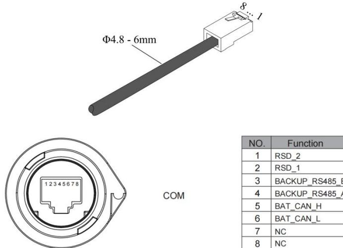
Step 2: Connect one end of the network cable to the corresponding port on the inverter.
