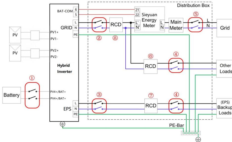
Note: All the home load can be connected to the EPS line as backup load, when the total amount of the load less than 6kW.
