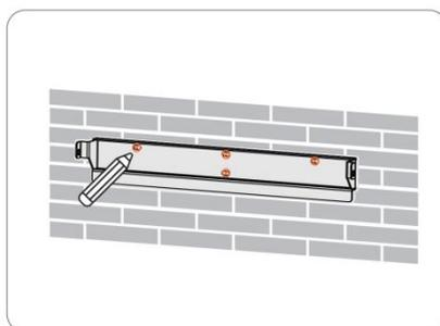
**Step 2** Use a hammer drill with a 10mm diameter drill bit to drill holes into the wall to a depth of 80mm.
