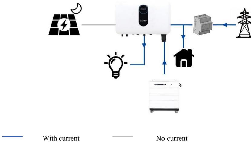
During night, when the battery is empty, it will enter into standby mode. In this case, the grid will supply all power for loads.
