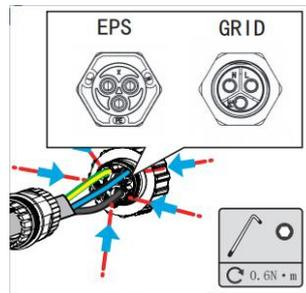
Step 4: Insert the terminals into the inverter grid socket.
