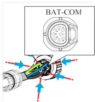
The following figure show the BAT-COM signal line position, where Pin1 connects to the battery CAN\_H, Pin2 connects to the battery CAN\_L, Pin3&Pin4 are connected to the battery 12V interface positive and negative (some batteries need to be connected to the 12V power supply, see the battery manual); Pin5&Pin6 are connected to the Sieyuan meter Pin21&Pin22. Pin7&Pin8 use for DO or Backup-RS485 (depending on the model).
