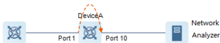
Figure 2-1 Operating Principle of Port Mirroring
