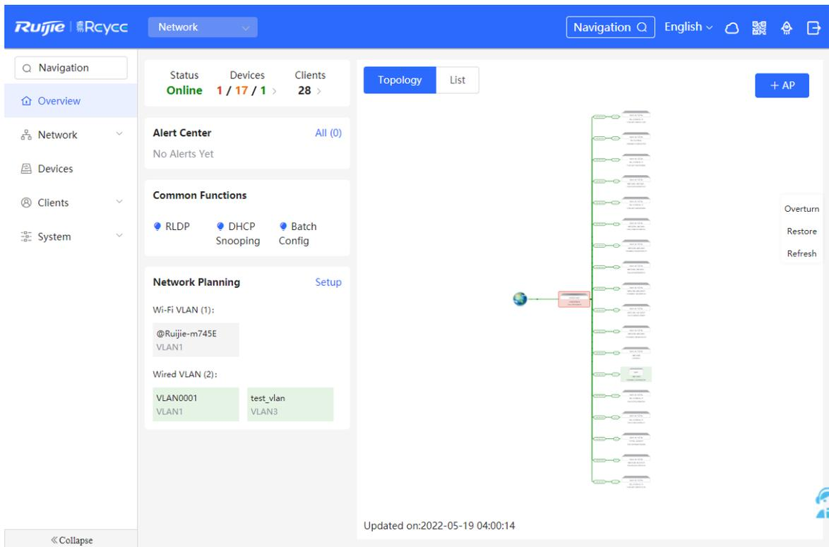
Figure1-3 The Web Page in Local Device Mode in Self-Organizing Mode
