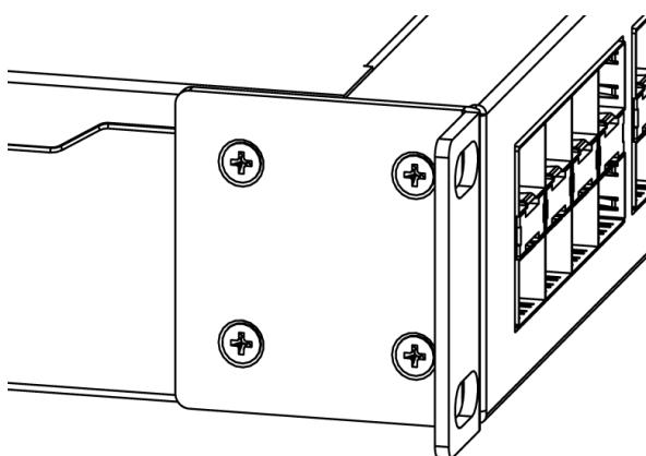
2. Place the device in a rackmount enclosure and align with the holes so that the device fits conveniently.
