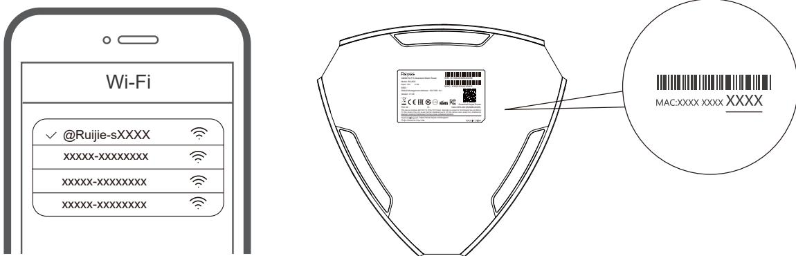
XXXX is the last 4 digits of the MAC address on the nameplate of router .
