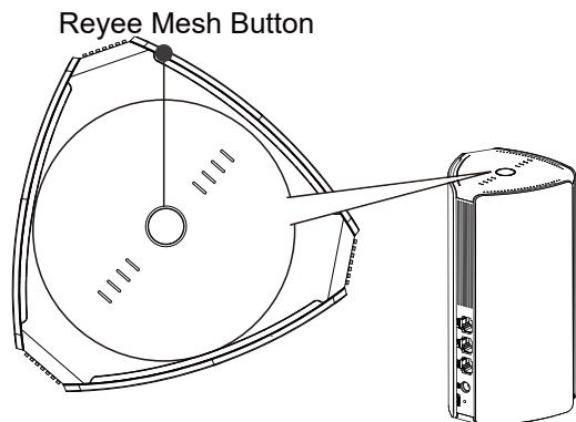
**4. Move the secondary router to an area where Wi-Fi coverage is required , and power it on again**
