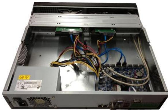
③ Connect to the HDD data cable to the main board and the HDD port respectively. Loosen the power cable of the chassis and connect another end of the power cable to the HDD port.
