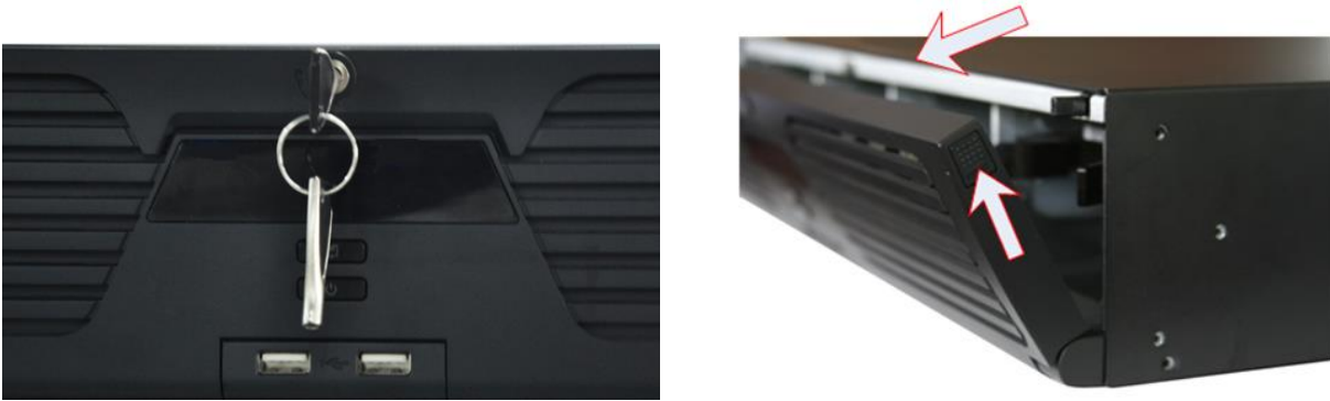
Figure 2-13 Open Front Panel
