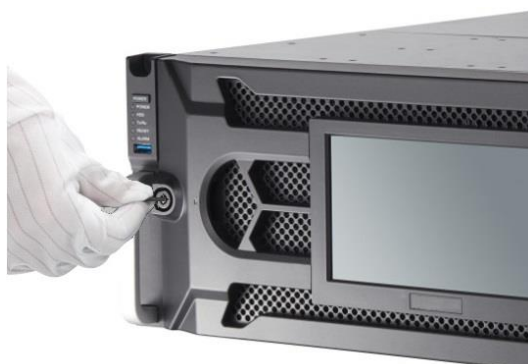
Figure 2-1 Unlock the Panel
