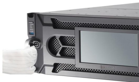
Figure 2-7 Reinstall the Cover and Lock the Panel
