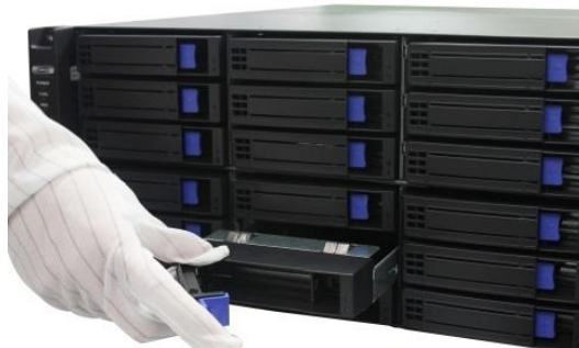
Figure 2-3 Pull out Dummy HDD
