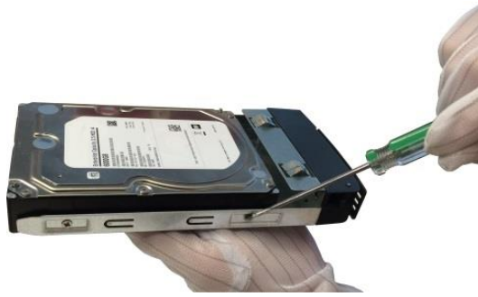
Figure 2-4 Fix the Hard Disk
