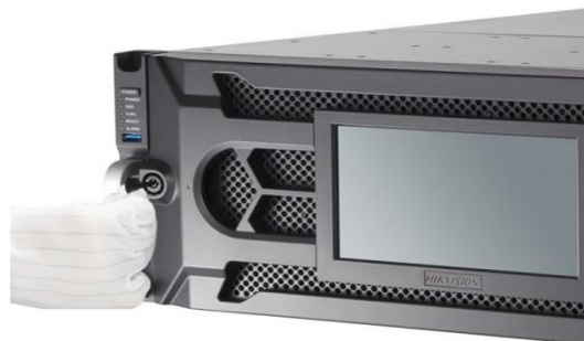
Figure 2-7 Reinstall the Cover and Lock the Panel
