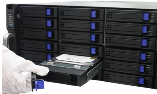
Figure 2-5 Push the Dummy HDD into the Slot
