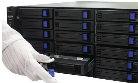
Figure 2-3 Pull out Dummy HDD
