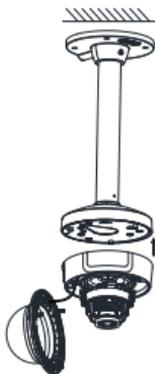
Figure 2-18 Secure the Camera
