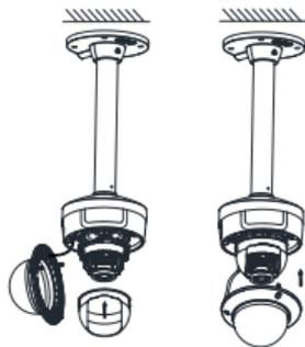
Figure 2-20 Secure Black Liner and Bubble
