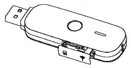
ii. Insert your microSD card into the microSD card slot, shown as the following picture.
