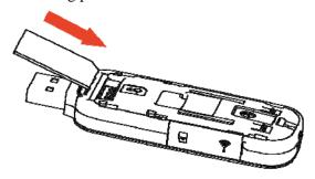
3. Put the front cover of the modem flatly upon the body of modem. Direct the front cover towards the locking catches on the sides of the modem, and then push the front cover of the modem to lock the front cover into its place.
